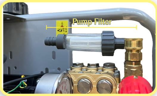
The pump filter protects the pump motor and other internal components from damage caused by dirt, sand, or other foreign particles. This helps the pump last longer and reduces the
